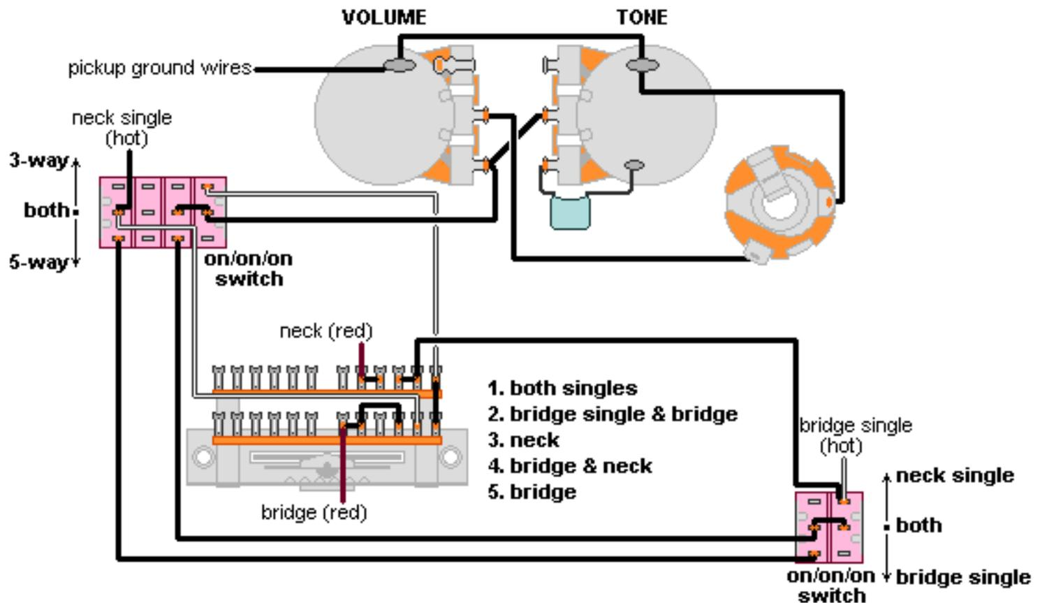
For Bridge and Neck, solder the black & white wires together and tape up each connection, green and bare is ground. All other pickup wires not shown or mentioned go to ground.
