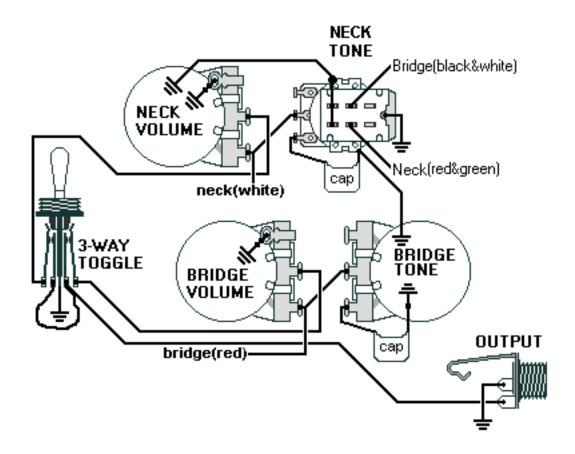
All other pickup wires not shown or mentioned go to ground. Note: Tailpiece should be connected to common ground. All grounds 🛓 must be connected.
