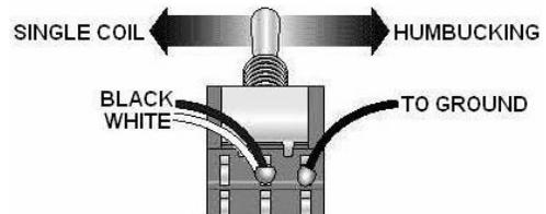
The **BARE** wire is always soldered to ground. As only one side of the DPDT mini-switch is used, you may choose to have two pickups go from double- to single-coil on one switch, like this:
