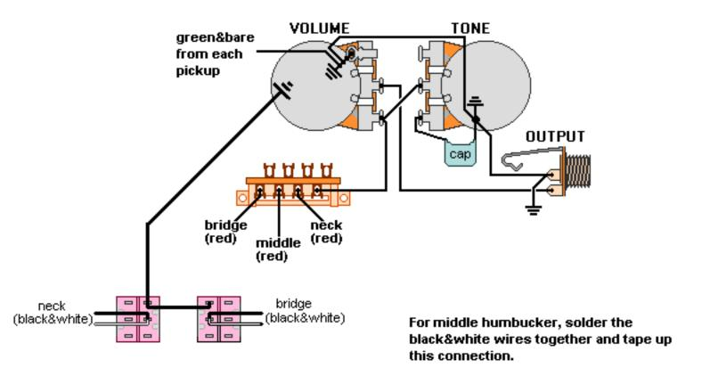
Note: Tailpiece should be connected to common ground. All grounds 🛓 must be connected.
