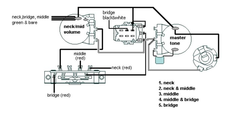
For eack pickup except bridge pickup, solder the black&white wires together and tape up each connection.
