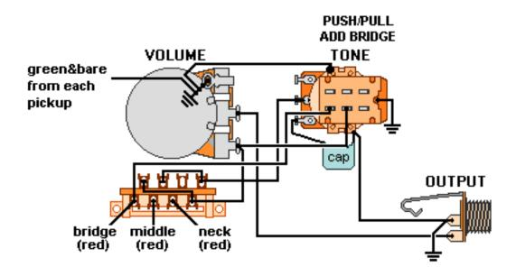
For each DiMarzio Humbucker, solder the black&white wires together and tape up this connection.
