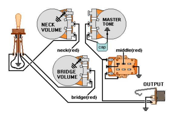
For each pickup, solder the black& white wire together and tape up the connection.
