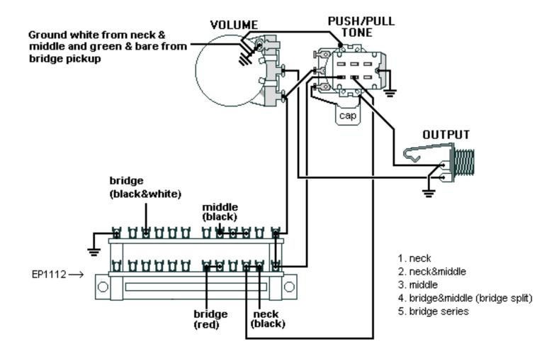
Note: Tailpiece should be connected to common ground. All grounds 🛓 must be connected.
