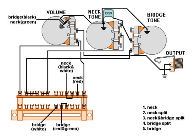
Note: Tailpiece should be connected to common ground. All grounds <u>L</u> must be connected.
