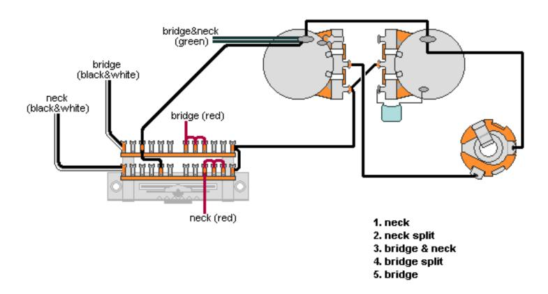
Note: Tailpiece should be connected to common ground. All grounds  $\underline{\bot}$  must be connected.
