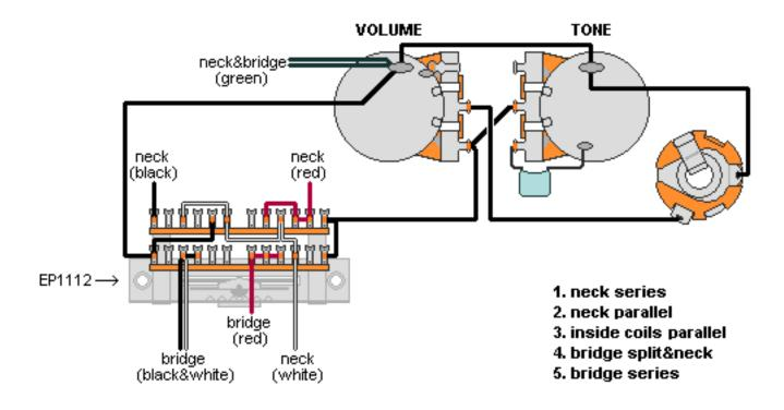
Both pickups should be installed with cable exits towards the controls
