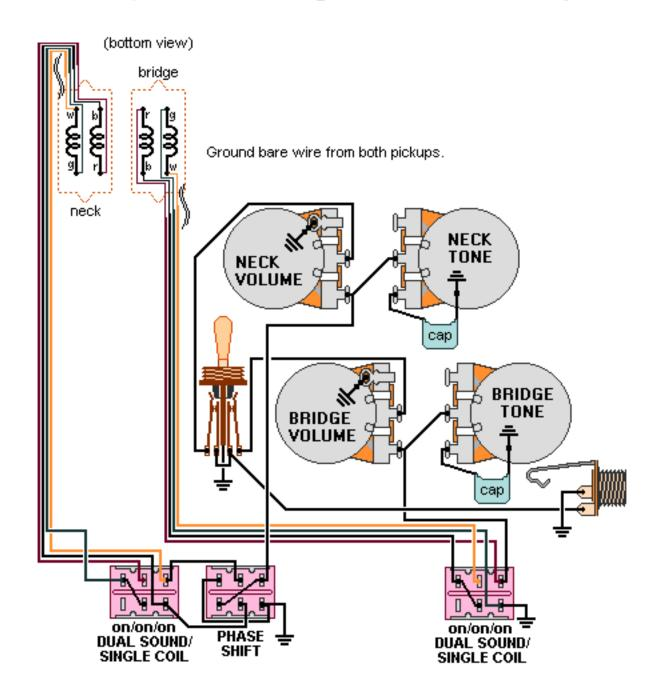
Note: Tailpiece should be connected to common ground. All grounds <u>+</u> must be connected.
