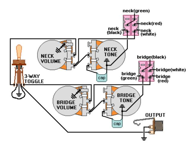
If both DPDT switches are on-on-on, the center position splits each pickup and cancels hum when both pickups are on
