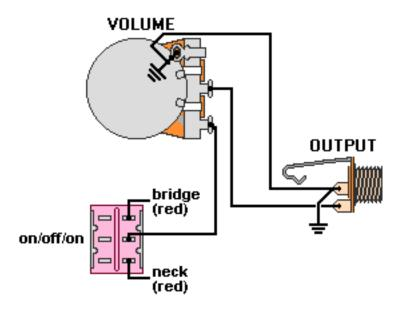
For each pickup, solder the black&white wires together and tape up this connection. Green&bare from each pickup goes to ground.
