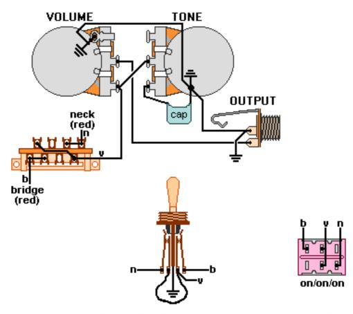
For each pickup, solder the black&white wires together and tape up this connection. The green and bare wires from both pickups go to ground.
