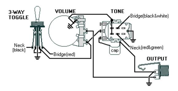
All other pickup wires not shown or mentioned go to ground. Note: Tailpiece should be connected to common ground. All grounds <u>L</u> must be connected.
