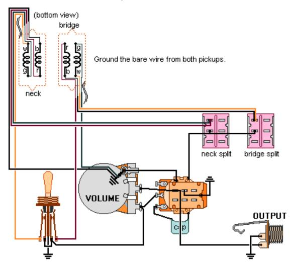
Note: Tailpiece should be connected to common ground. All grounds 🛓 must be connected.
