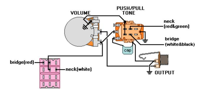
The neck pickup should be installed with the cable exit away from the controls. Install the bridge pickup with the cable exit towards the controls.
