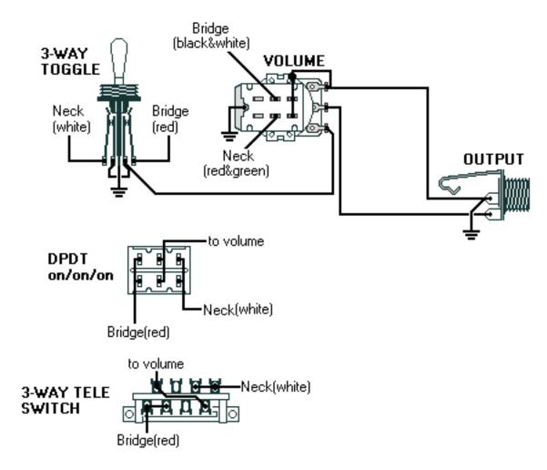
Install both pickups with cable exits towards bridge
