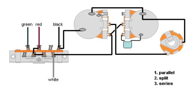
Note: Tailpiece should be connected to common ground. All grounds  $\c \bot$  must be connected.
