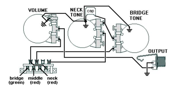
neck & middle pickups - for each pickup, solder the black&white wires together and tape up the connections. Ground the green & bare wires.
