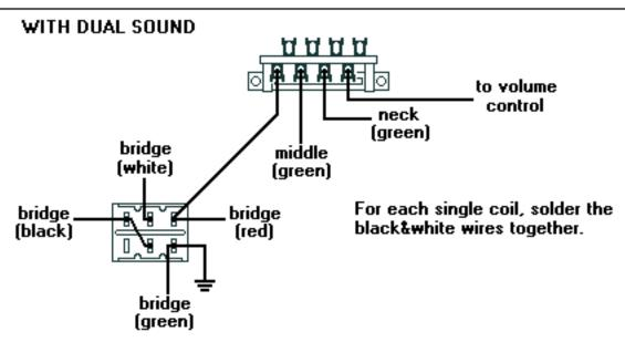
All other pickup wires not shown or mentioned go to ground. Note: Tailpiece should be connected to common ground. All grounds <u>L</u> must be connected.
