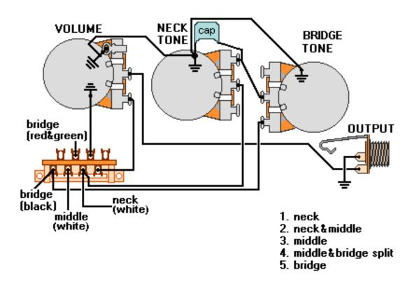
All other pickup wires not shown or mentioned go to ground. Note: Tailpiece should be connected to common ground. All grounds 🛓 must be connected.
